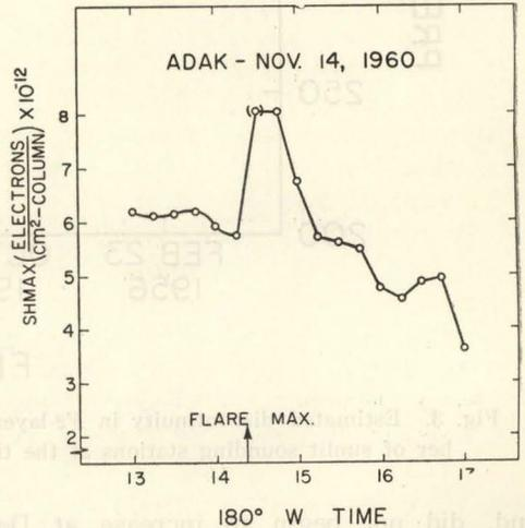
Fig. 6. Sub-peak electron content at Adak during November 15 flare event.
