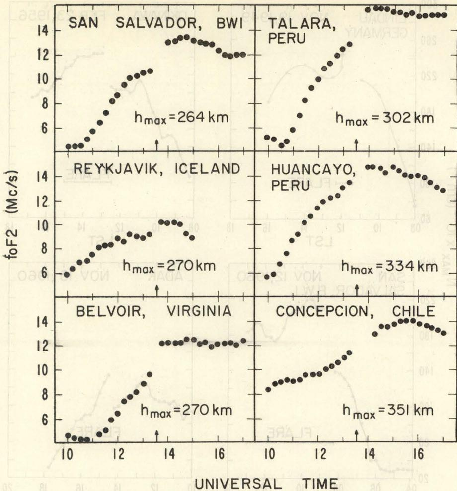
Fig. 2. Variations in  $F_2$ -layer penetration frequency at six sunlit sounding stations during the large solar flare of November 12, 1960. Arrow marks flare beginning.
