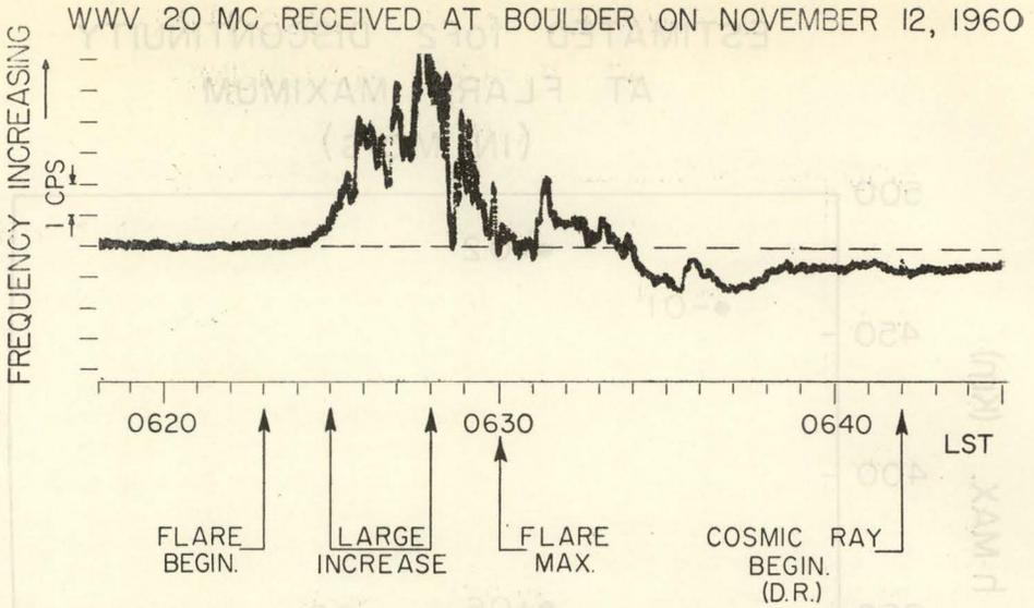
Fig. 4. Variations in the frequency of WWV 20 Mc/s signal as recorded at Boulder, Colorado, November 12, 1960, 105°W time.
