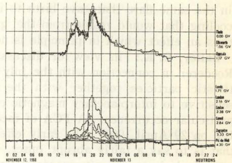
Fig. 24. Observations on Nov. 12 and 13, 1960, at different stations selected to show the progressive breakdown of the geomagnetic cutoff beginning at 1700 UT on Nov. 12.
