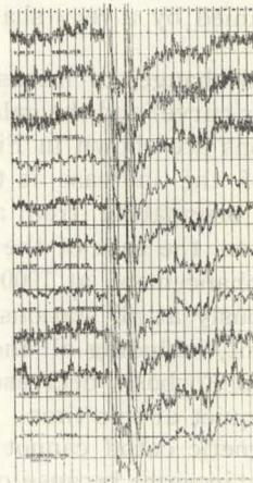
Fig. 17. Nov. 1960 neutron monitor observations from ten stations in North America. The Nov. 12 and Nov. 15 solar particle events go off-scale on these plots which are scaled to exhibit the Forbush decrease. The solar particle event of Nov. 20 can be seen at each of these stations.
