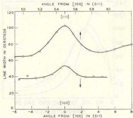
Fig. 3. Line width versus angle near [111] and [100] for YIG (0.02% Tb) as measured at 23°K. The frequency was 20.8 kMc/sec.
