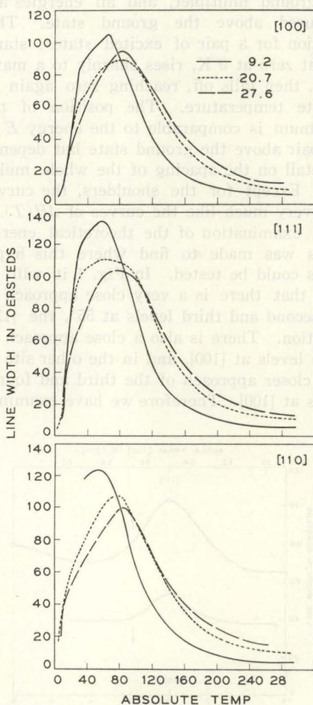
Fig. 2. Line width plotted against temperature for YIG (0.02%Tb) with the field along each of the principal crystallographic directions. Data taken at 9.2, 20.7, and 27.6 kMc.
