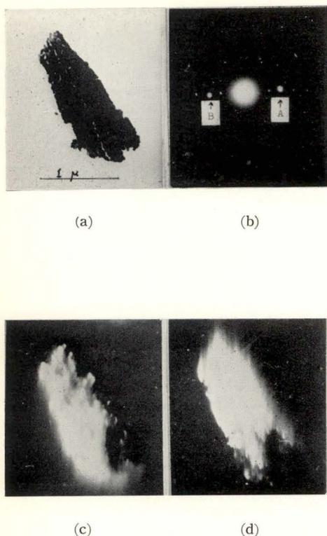
Fig. 1. (a) Electron microphotograph and (b) diffraction photograph of  $\alpha$ - $\text{Fe}_2\text{O}_3$  obtained by the calcination of  $\text{Fe}(\text{NO}_3)_3 \cdot 9\text{H}_2\text{O}$  at  $500^\circ\text{C}$  for 2 hrs. (c), (d) Dark field image photographs of corresponding diffraction patterns of A and B in (b).
