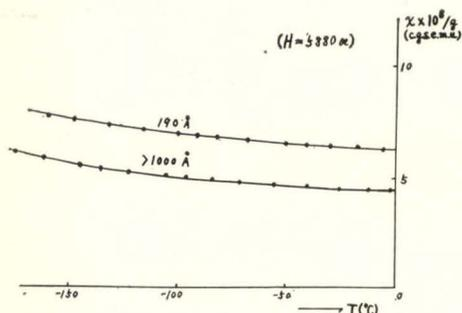
Fig. 7.  $\chi$ - $T$  curves of  $\text{V}_2\text{O}_4$ .
