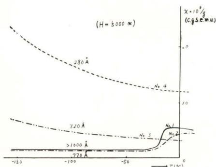
Fig. 4.  $\chi$ - $T$  curves of  $\alpha$ -Fe<sub>2</sub>O<sub>3</sub> prepared from Fe(NO<sub>3</sub>)<sub>3</sub>·9H<sub>2</sub>O.
