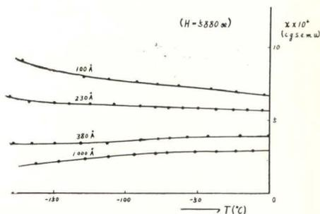
Fig. 6.  $\chi$ - $T$  curves of CuO prepared from Cu(OH)<sub>2</sub>·CuCO<sub>3</sub>.
