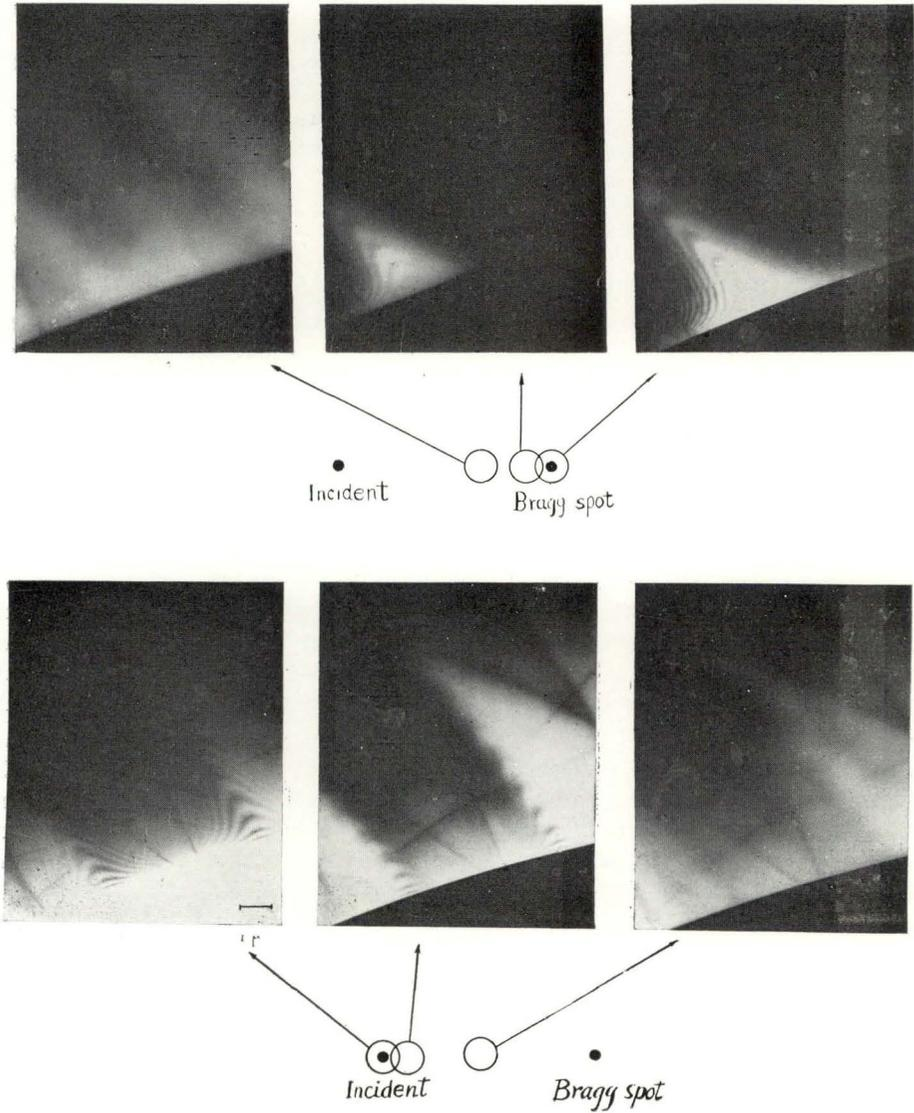
Fig. 3. Extinction contours of aluminum crystal. Pictures taken at various positions of objective aperture.
