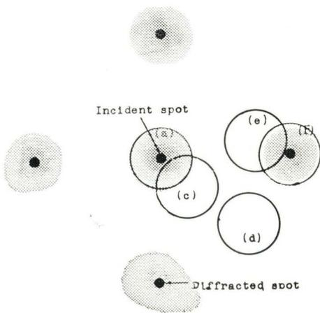
Fig. 1. Various positions of objective aperture (a) Bright field (with the incident spot), (b) Usual dark field (with a diffraction spot), (c), (d) and (e) Special dark field (without any diffraction spot).
