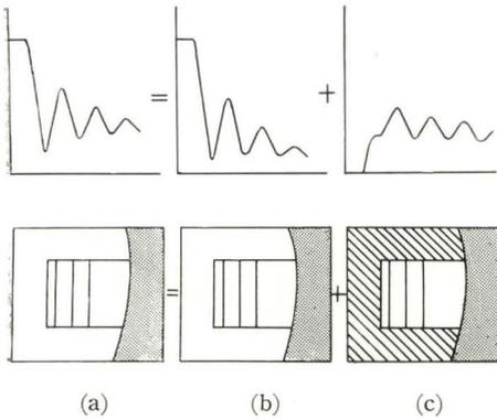
Fig. 4. Illustrating the nature of bright field image. A bright field image (a) is the superposition of c-image (b) and i-image (c).
