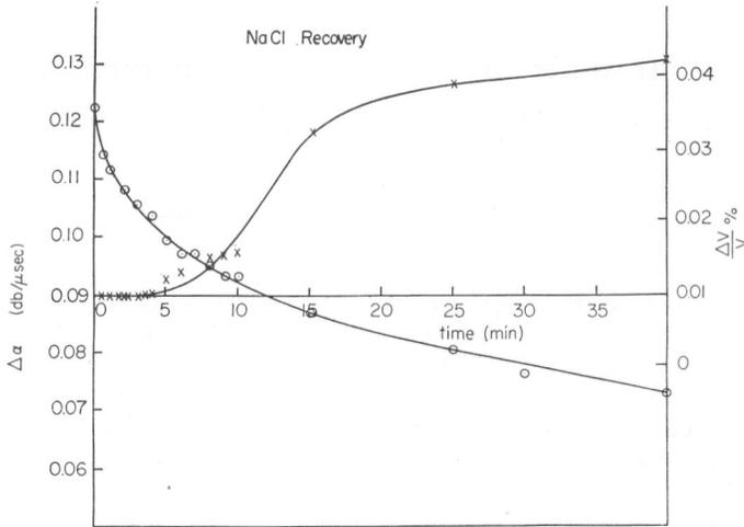
Fig. 5. Recovery of ultrasonic attenuation and velocity in slightly deformed NaCl observed with 10 mc/sec  $\langle 100 \rangle$  compressional waves. Unpublished measurements of Hikata *et al.*
