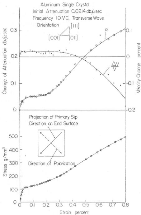
Fig. 3. Stress, shear wave attenuation and velocity change as a function of total strain in aluminum. Hikata *et al.*
