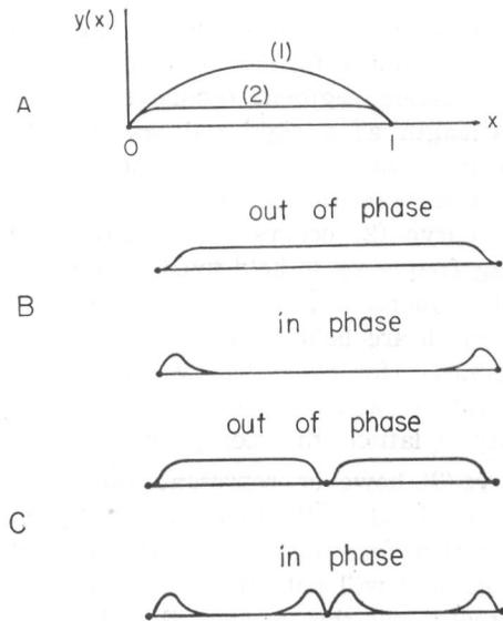
Fig. 1 Displacement of a dislocation under stress (Schematic)
