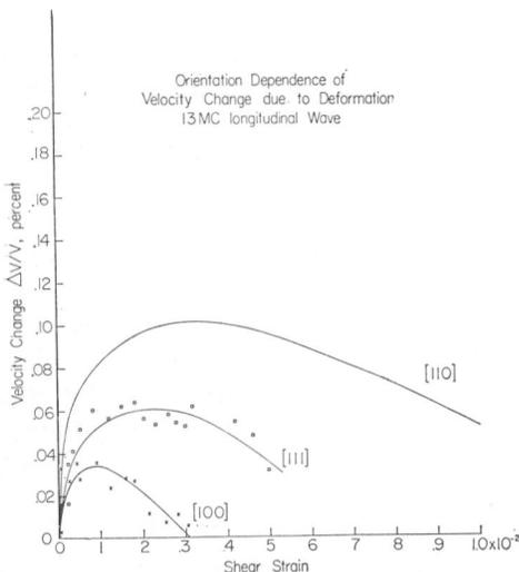
Fig. 4. Longitudinal wave velocity change  $\Delta v/v$  for  $\langle 100 \rangle$ ,  $\langle 111 \rangle$  and  $\langle 110 \rangle$  orientation as a function of shear strain. Hikata *et al.*
