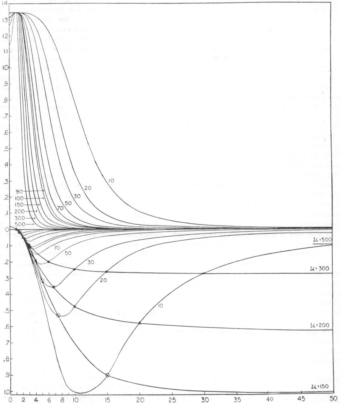
Fig. 2. Normalized attenuation and ultrasonic velocity change for a solid containing dislocations as a function of normalized dislocation resonant frequency  $\gamma = \omega_0/\omega$ .
