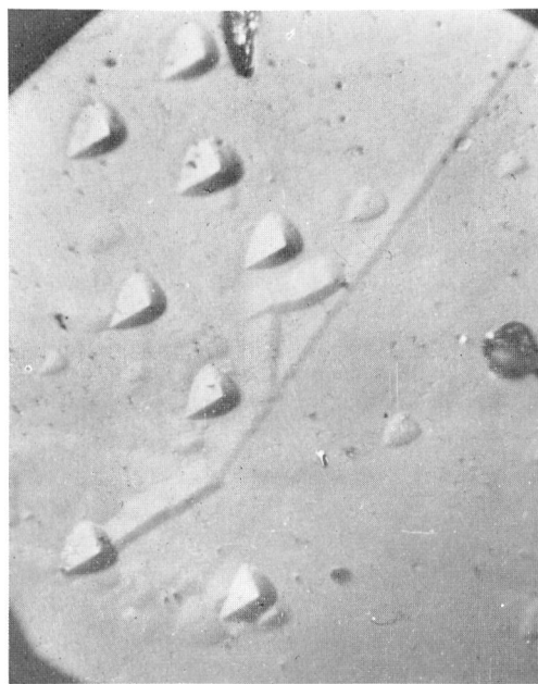
Fig. 7. Clusters of point defects in the twin. \times 600 .
