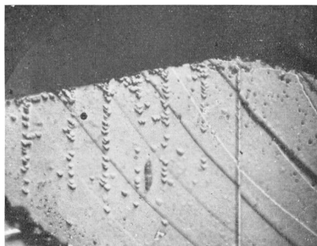
Fig. 6. Rows of dislocations at the places of stoppage of the twin boundary. \times 340 .
