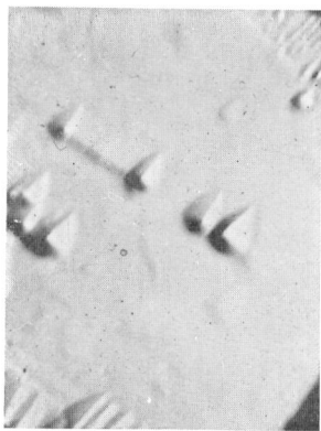
Fig. 5. Stacking fault in twin of calcite crystal. \times 600 .
