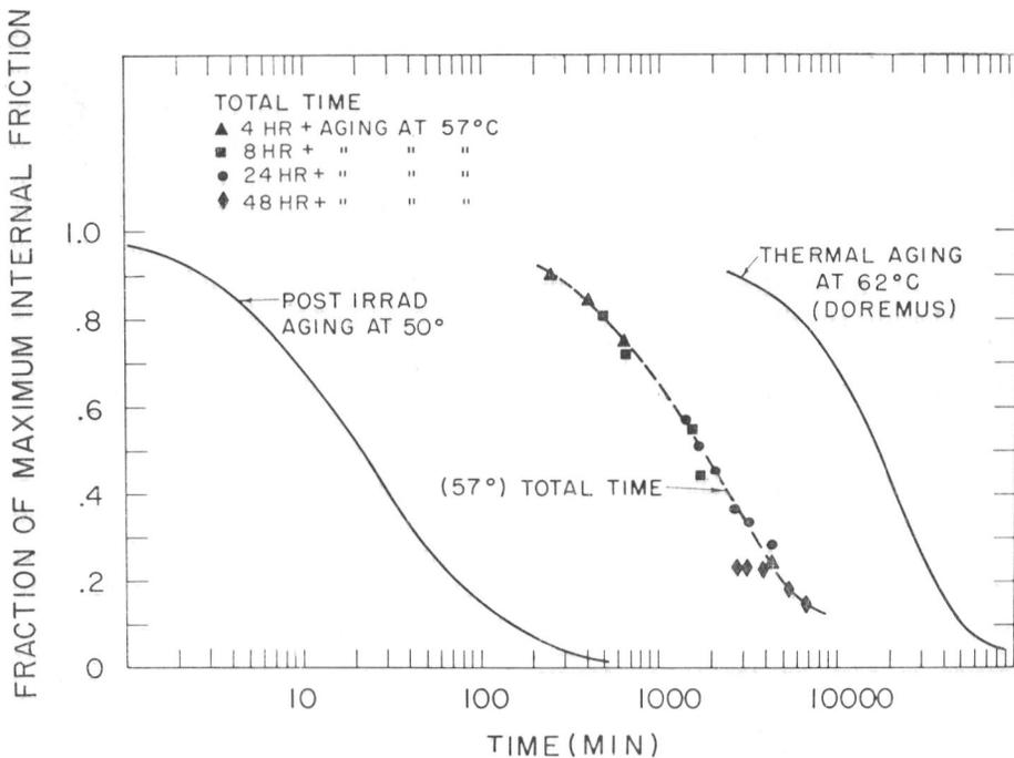
Fig. 1. Summary of internal friction studies of carbon in iron. Right curve—thermal rate (Ref. 1). Middle curve—irradiation and aging at  $57^\circ\text{C}$ . Left curve—aging at  $50^\circ\text{C}$  after irradiation at  $-100^\circ\text{C}$  (Ref. 2).
