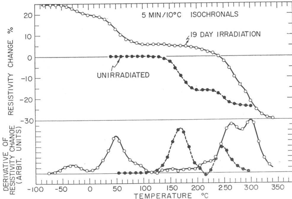
Fig. 3. Resistivity and temperature derivative of resistivity during isochronal annealing of iron-carbon irradiated for 19 days at  $-100^{\circ}\text{C}$  compared with an unirradiated specimen.
