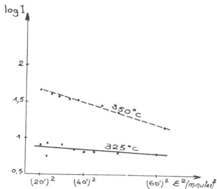
Fig. 3. Small angle scattering given by a crystal annealed for 1 hour at 325°C and 350°C.
