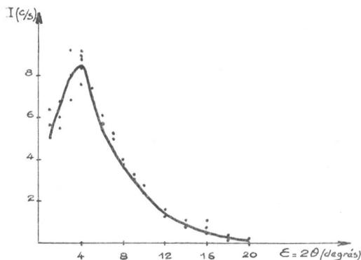
Fig. 1. Scattered intensity (room temperature).
