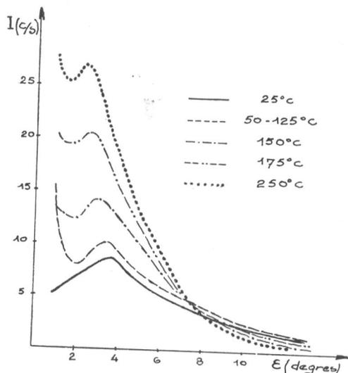
Fig. 2. Displacement of the scattering curve during the annealing of the crystal.
