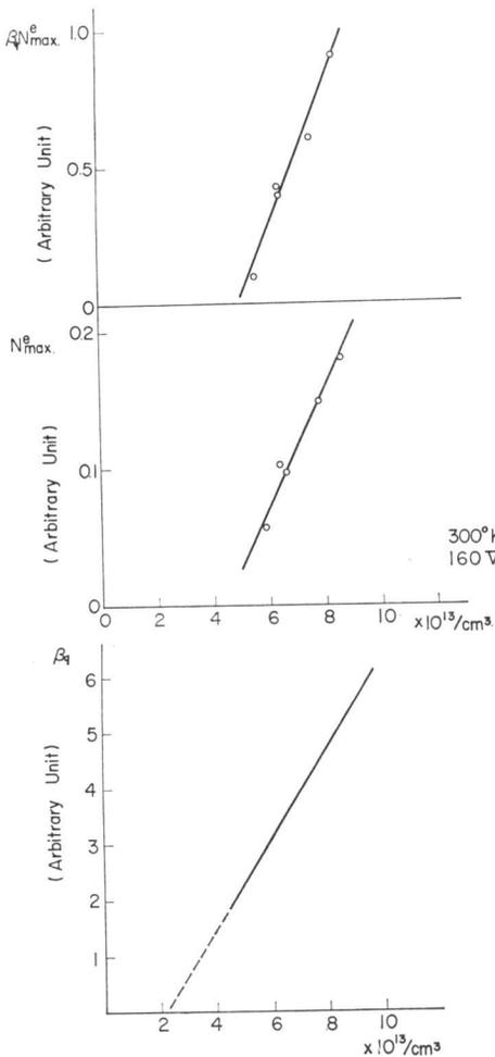
Fig. 3. Observed carrier density dependence of decay constant  $\beta_q$ . Experiments were performed at room temperature. Carrier density  $n$  was estimated from the Ohmic conductivity, assuming  $\mu=260 \text{ cm}^2/\text{V sec}$ .
