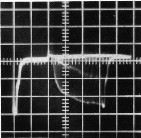
Fig. 1(b). Multiply exposed photograph of the above double pulse oscilloscope traces. The interval was changed up to about 6  $\mu$  sec manually.
