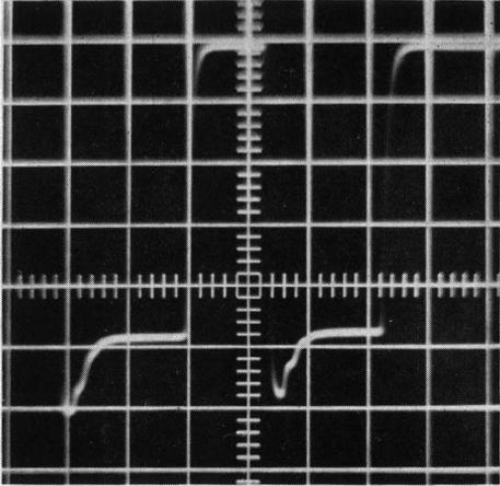
Fig. 1(a). Oscilloscope trace of a pair of current pulses. Time runs from left to right. The second pulse is applied 3  $\mu$  sec later than the first one.
