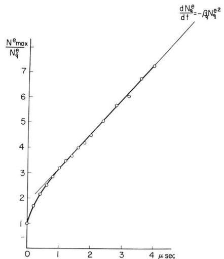
Fig. 2. Observed  $N_{q^e}^{\max}/N_q^e(t)$  versus  $t$  curve. The solution of eq. (6),  $N_{q^e}^{\max}/N_q^e(t) - 1 = \beta_2 N_{q^e}^{\max} t$  is compared with the observations. The initial condition here is taken to be at the end of the first pulse.
