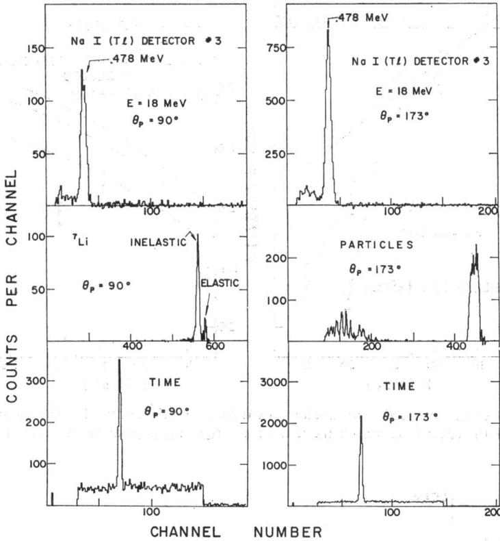
Fig. 2. Energy spectra of gamma rays, particles and their time relationship, observed in coincidence at  $\theta_p = 90^\circ$  and  $173^\circ$ .
