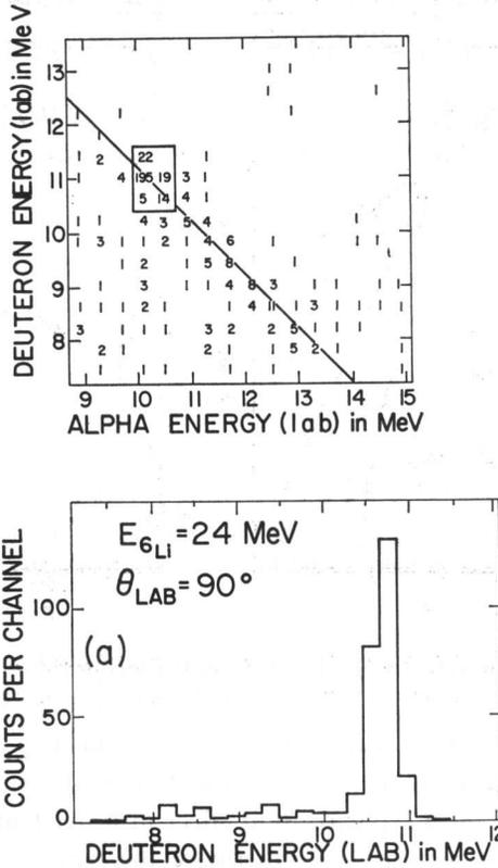
Fig. 5. Upper half: Two dimensional spectra of  $\alpha$  and deuteron energies observed at  $E_{Li} = 24 \text{ MeV}$ . Lower half: deuteron spectrum obtained after summation along the kinematic line shown in the upper spectrum.
