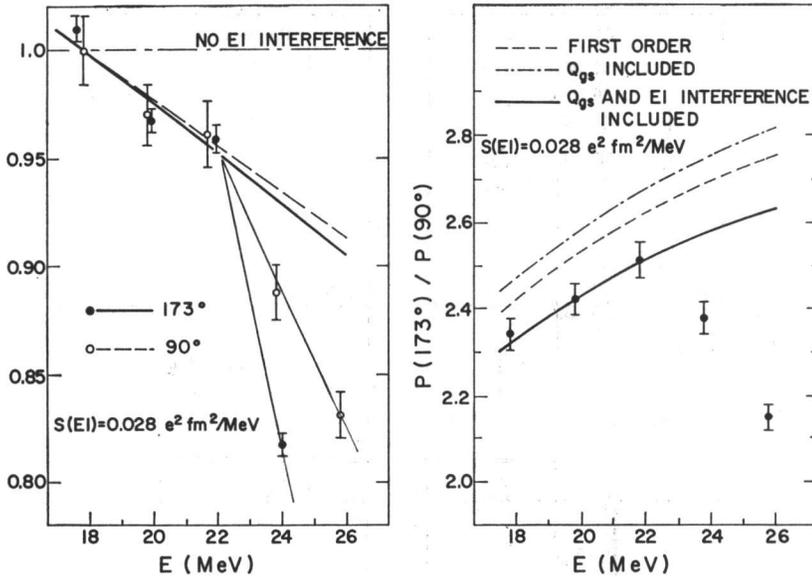
Fig. 3. Effect of EI polarization on Coulomb excitation probabilities in  $^7\text{Li}$ . The linear energy dependence of the effect is shown on the left. On the right the angular dependence of the effect is shown.
