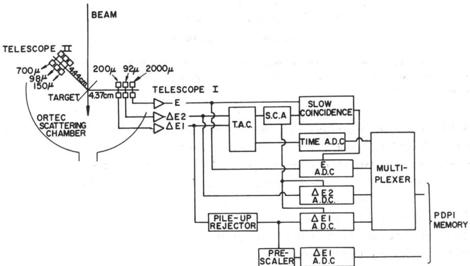
Fig. 4. Experimental arrangement used to study the Coulomb breakup of  $^6\text{Li}$ .
