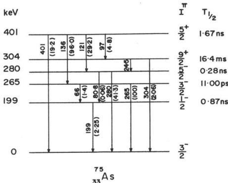
Fig. 1. Partial level scheme of <sup>75</sup>As levels populated in the decay of <sup>75</sup>Se.
