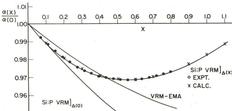
Fig. 2 Calculated  $\alpha_D(x_{100})/\alpha_D(0)$  versus  $x$  compared with Si:P data
