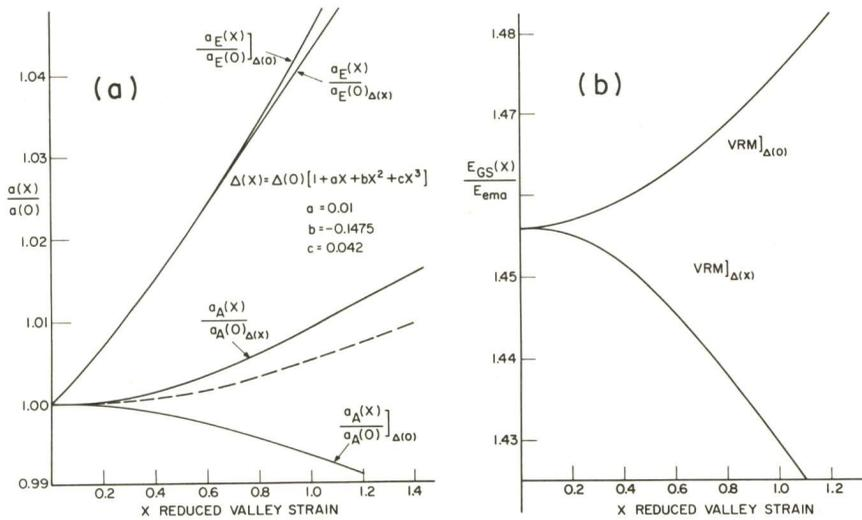
Fig. 3 Bohr radii  $a_A(x)$  and  $a_E(x)$  and energy  $E_{GS}(x)$  vs.  $x$  for Si:P
