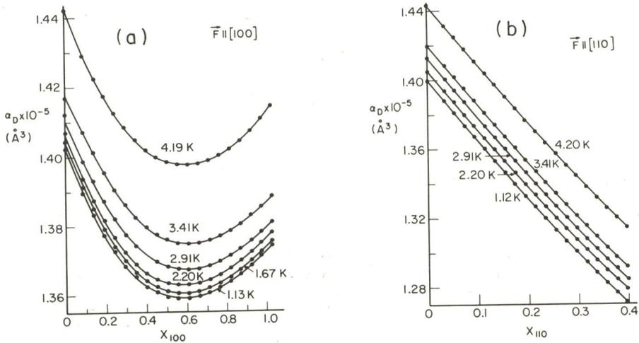
Fig. 1  $\alpha_D(x)$  versus  $x$  for Si:P ( $N_D \sim 5 \times 10^{17}/\text{cm}^3$ ), a) [100], b) [110]
