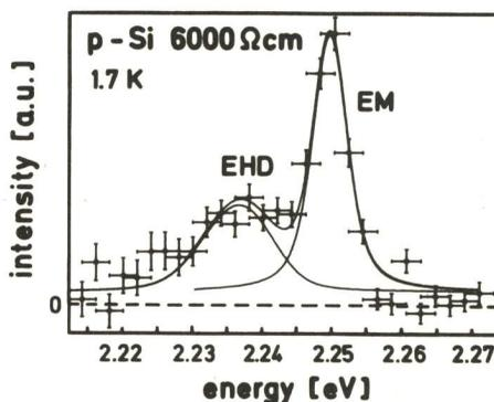
Fig. 4 Emission spectrum of Si[2;1] near  $2E_g$ : The EM line is much stronger than in Fig. (2)
