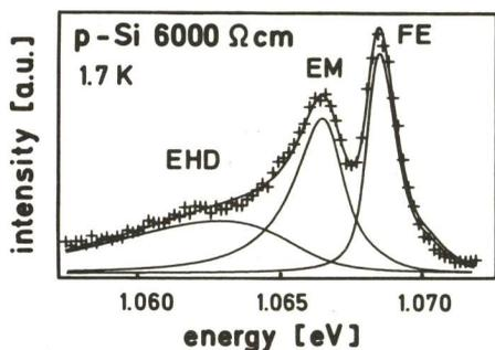
Fig. 3 Luminescence spectrum of Si[2;1] in the high stress limit: The drawn line shape is composed of EHD, EM, and FE
