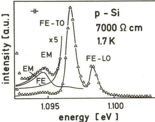
Fig. 1 FE and EM emission near the band gap energy of Si[6;2]: The drawn lines represent calculated line shapes
