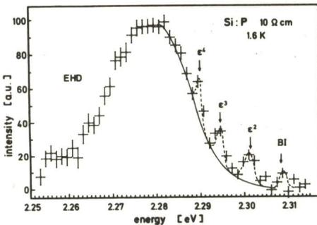
Fig. 2 Emission spectrum of Si[6;2] near  $2E_g$ : The labels are defined in the text
