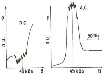
Fig.4 Longitudinal photoconductivity vs. magnetic field for  $Cd_{1-x}Mn_xSe$  ( $x = 0.001$ ) at 4.2K ( $\hbar\omega = 0.5$  meV): DC measurement is shown on the left hand side, AC measurement ( $f = 1KHz$ ) - on the right hand side
