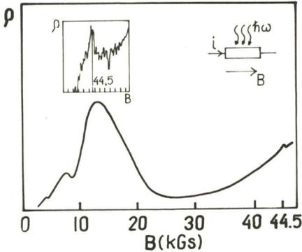
Fig.2 Longitudinal photoconductivity vs. magnetic field for  $\text{Hg}_{1-x}\text{Mn}_x\text{Te}$  / $x = 0.003$ / at 4.2K: The incident light energy  $\hbar\omega = 0.5\text{meV}$ , current through the sample  $i = 10\mu\text{A}$ . Resonance peak is enlarged in the insert
