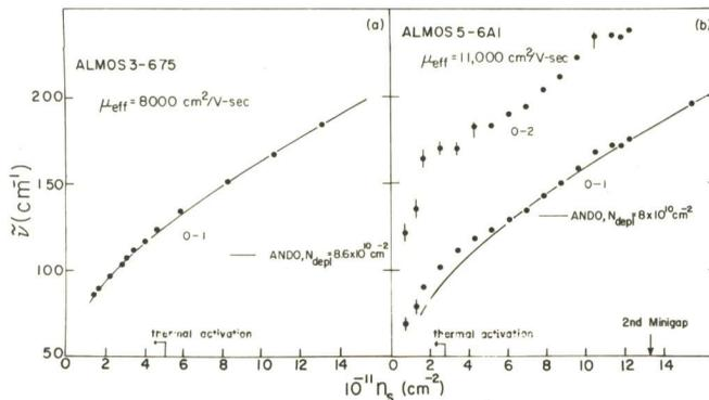
Figure 1 Intersubband transition energies as a function of carrier density for two samples: Solid curves are theoretical results of Ando for two valley occupancy
