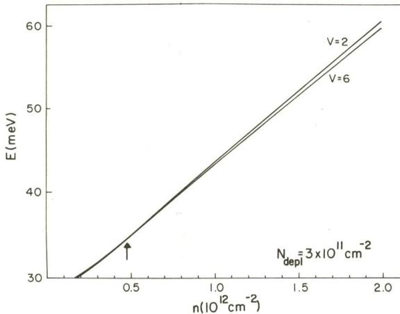
Figure 2 Total ground state energy per particle for six and two valley occupancy vs. density: The arrow indicates the critical density
