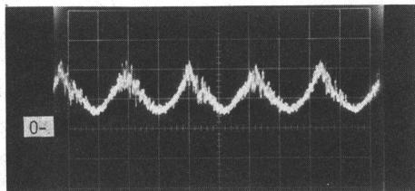
Fig. 2. Current pattern observed during the electrostatic rotation of the  $\text{LiNbO}_3$  rotor in an atmosphere (R.H = 76%).
