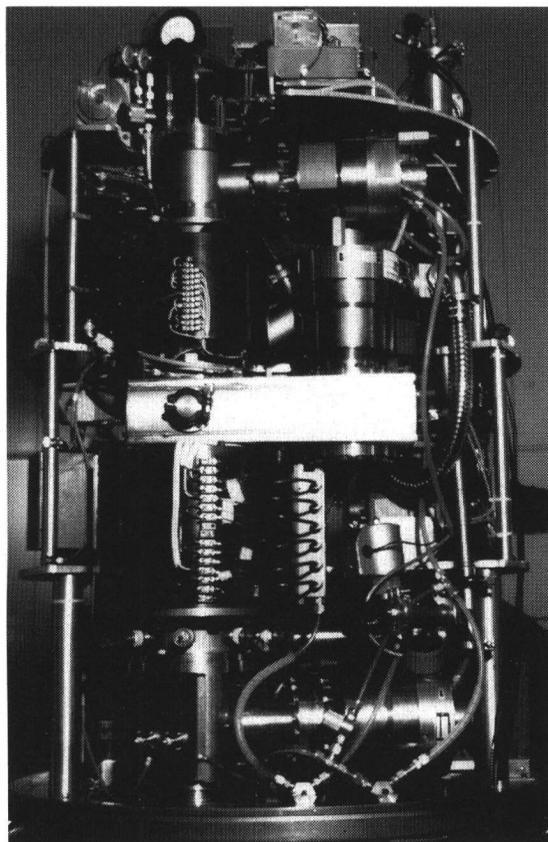
Fig. 3 · Polarized  $^3\text{He}$  ion source installed in the terminal of the CN van de Graaff.
