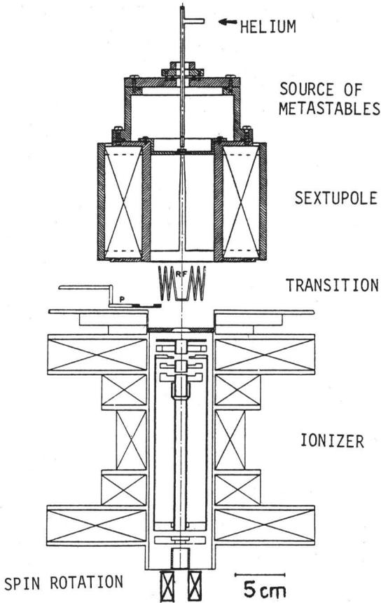
Fig. 2. Schematic of the source (pumping systems not shown)
