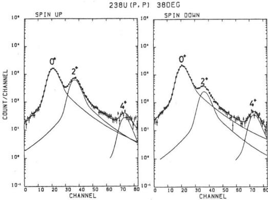
Fig. 1 Typical result of the peak fit. Spin up spectrum and spin down one are fitted simultaneously with same peak shape and position parameters.
