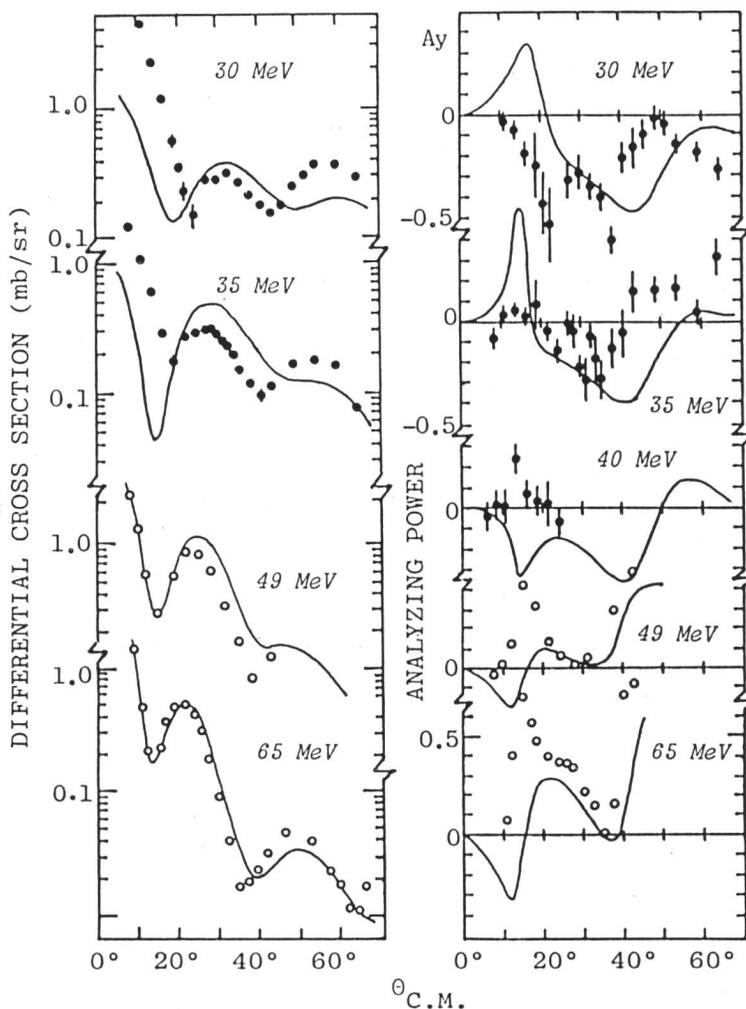
Fig. 1. The angular distributions of the differential cross sections and the analyzing powers for the  $^{24}\text{Mg}(p, d)^{23}\text{Mg}$  reaction to the 2.36 MeV,  $l=0; 1/2^+$  state at 30, 35 and 40 MeV. The data at 49 and 65 MeV of Refs. 3) and 2), respectively, are also shown for comparison. The solid lines show the preliminary DWBA calculations using the same optical potential parameters used by K. Hatanaka *et al.* <sup>2)</sup>.
