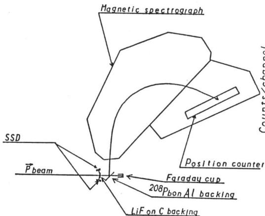
Fig. 1. Schematic view of the counter system.
