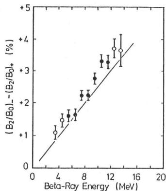
Fig. 2. Difference of  $B_2/B_0$  for  $^{12}\text{B}$  and  $^{12}\text{N}$ . Closed circles are data used for the analysis. Solid line is theoretical one<sup>4)</sup>.
