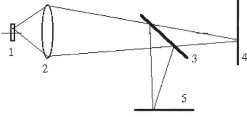
Fig.2. The scheme of a phase-contrast neutron microscope; 1 : spin-flipper with object placed inside, 2 : objective, 3 : analyzer-splitter for neutron beam, 4, 5 : 2D-detector.
