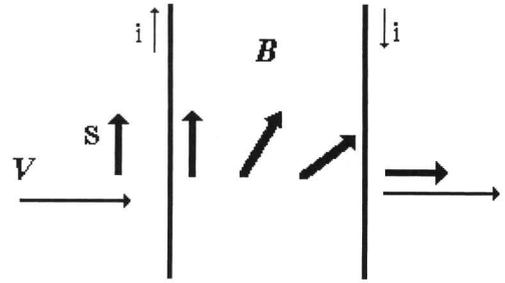
Fig.1. The spin-flipper scheme;  $B$ : magnetic field,  $V$ :neutron velocity,  $S$ : neutron spin,  $i$ : foil current.
