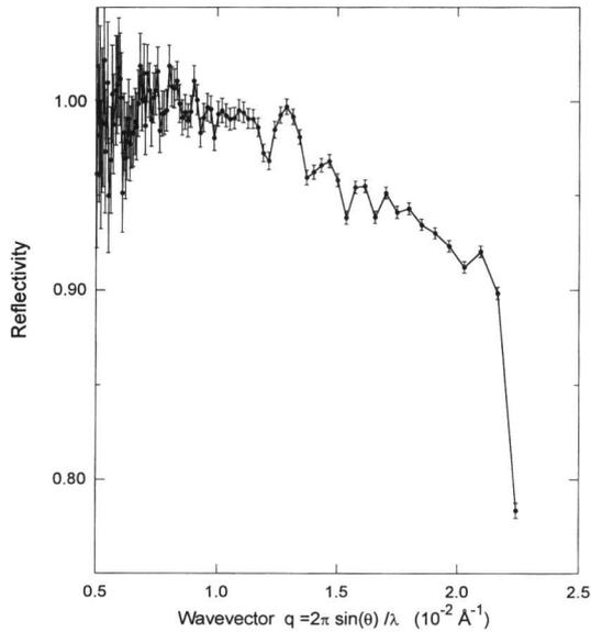
Fig. 1. Measured reflectivity for one of the supermirrors used for G3-bis.
