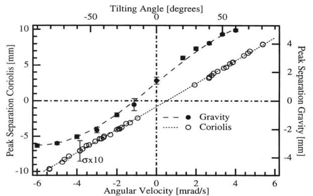
Fig. 3. Fig. 2: Peak separation as a function of the tilting angle (Gravity) and angular velocity (Coriolis).
