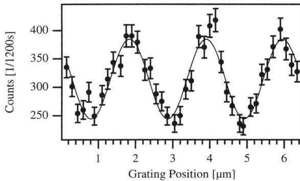
Fig. 4. Interference fringes measured with the VCN interferometer. The distance of the phase gratings was 25cm. The straight line is the result of a fit with the function  $f(x) = U + A \cdot \sin(2\pi x/d + \varphi_0)$ , with  $d$  being the spacing of the gratings of  $2\mu\text{m}$
