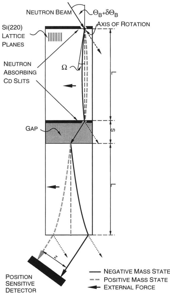
Fig. 1. Neutron trajectories in the gravity experiment.. The fine dashed lines are the neutron trajectories without external force; the fat line trajectories are valid with external force. The dimensions were  $L = 52.3\text{mm}$  and  $s = 9.6\text{mm}$ . The arrangement of the slits and the neutron trajectories in the Coriolis experiment can be found in Ref.4. The slit width was 1.6 mm in the Coriolis experiment and 1.5 mm in the gravity experiment.
