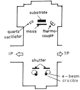
Fig. 1. The schematic of the vacuum deposition unit. TP denotes turbomolecular pump and IP denotes ion pump.
