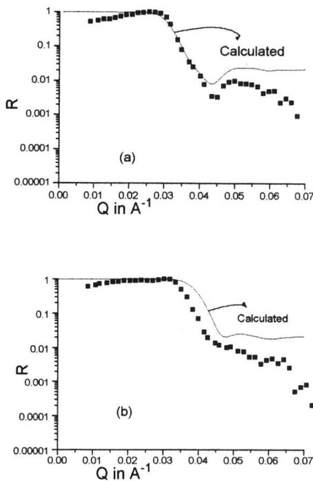
Fig.4. (a) The measured reflectivity,  $R$  (circles) vs.  $Q$  for the mirror with 10 bilayers and the ideal calculated profile (continuous line); (b) Measured  $R$  (circles) and ideal calculated (continuous line) for the mirror with 30 bilayers.
