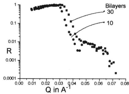
Fig.3. Reflectivity ( $R$ ) plotted against  $Q$  for both the supermirrors. The mirror with 10 bilayers has a critical angle of 36 minutes of an arc and the mirror with 30 bilayers has a critical angle of 41 minutes of an arc.
