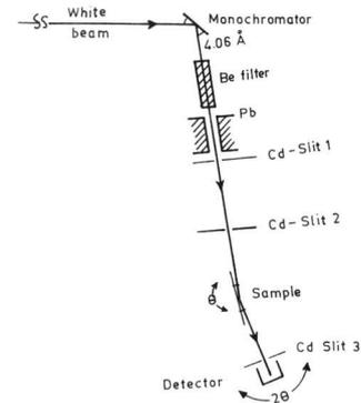
Fig.2. The neutron reflectometer setup at Dhruva. The monochromator used is pyrolytic graphite, giving 4.06 Å neutrons. The lead block with a slit of about 5mm × 35mm is used to reduce the gamma background. Beryllium filter is used to remove 2 Å neutrons from the beam. Cd slit 1 and Cd slit 2 are the cadmium slits which form the collimator, giving a beam of 6 minutes of arc divergence.
