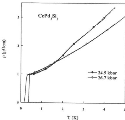
Fig. 7. Temperature dependence of the resistivity  $\rho$  just below the QCP and at the QCP.
