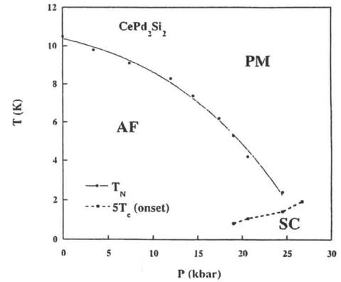
Fig. 5.  $(T, P)$  phase diagram of  $\text{CePd}_2\text{Si}_2$ . The full line describes the AF - PA boundary, the dashed line shows the superconducting (SC) boundary. For clarity, the  $T_c$  value has been multiplied by 5.
