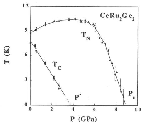
Fig. 2.  $T, P$  phase diagram of  $\text{CeRu}_2\text{Ge}_2$  after reference (43). The second order transition line separates the paramagnetic (PA) and antiferromagnetic (AF) phases; the first order transition line is between the AF and ferromagnetic phases. At  $T = 0$ , the respective characteristic pressures are  $P_c$  and  $P^*$ . similar results were obtained in the reference (44, 45).
