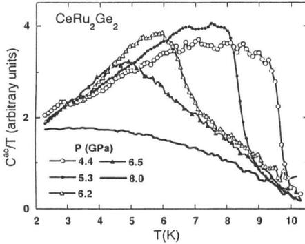
Fig. 4. Specific heat anomaly of  $\text{CeRu}_2\text{Ge}_2$  measured below the QCP using ac calorimetry and the new clean pressure system described in the text.
