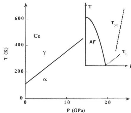
Fig. 1.  $T, P$  phase diagram of metallic cerium. The continuous line is the first order  $T_{\gamma\alpha}(P)$  transition line: long range magnetic ordering cannot appear in the intermediate valence  $\alpha$  phase. The insert shows the opposite situation where antiferromagnetic ground state occurs below the QCP at  $P = P_c$ ; Fermi liquid properties in the paramagnetic state can be observed only below  $T_I$ .
