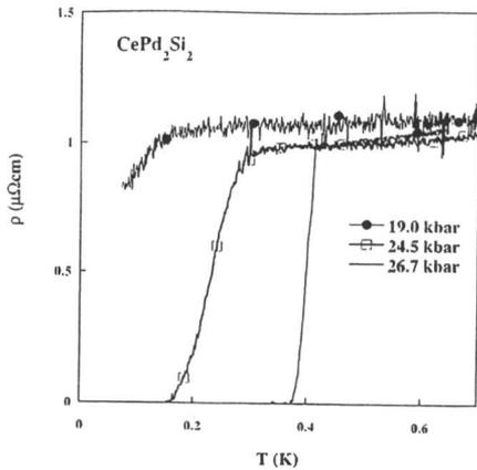
Fig. 6. Resistivity superconducting drops of  $\text{CePd}_2\text{Si}_2$  below the QCP for three different pressures.
