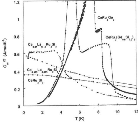
Fig. 3. Temperature variation of  $C/T$  (from reference (42)) measured in  $\text{CeRu}_2\text{Ge}_2$  at  $P = 0$  and data obtained on alloying systems  $\text{CeRu}_2(\text{Ge}_{1-x}\text{Si}_x)_2$  and  $\text{Ce}_{1-x}\text{La}_x\text{Ru}_2\text{Si}_2$ .
