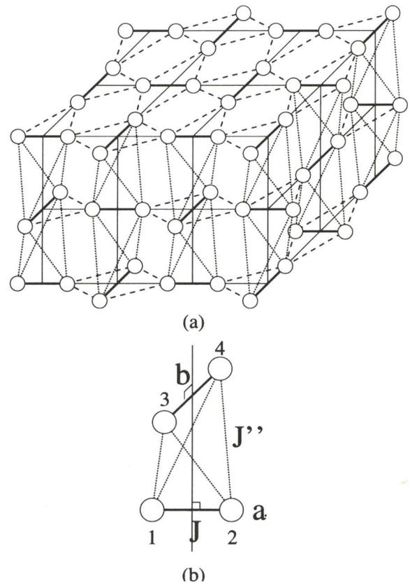
Fig. 4. (a) The model for  $\text{SrCu}_2(\text{BO}_3)_2$ : Three-dimensional orthogonal dimer model. (b) The configurations of two dimers along the  $c$ -axis are also orthogonal in a different way from Fig. 2(b).
