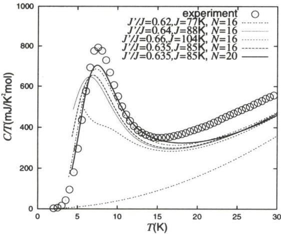
Fig. 8. The temperature dependence of the specific heat of  $\text{SrCu}_2(\text{BO}_3)_2$ . The fit parameters are  $J = 85$  K,  $J' = 54$  K.  $0.4 \times T^3$  is used as the contribution from phonon degrees of freedom.
