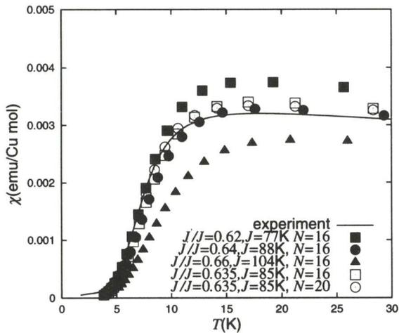
Fig. 5. The temperature dependence of the magnetic susceptibility on the two-dimensional model.  $J'/J = 0.62$ ,  $J''/J = 0.64$ ,  $J'/J = 0.635$ , and  $J''/J = 0.66$ .
