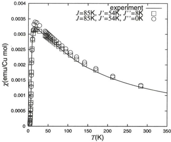
Fig. 7. Fit of the uniform magnetic susceptibility for  $\text{SrCu}_2(\text{BO}_3)_2$ . The parameters used are  $J = 85$  K,  $J' = 54$  K, and  $J'' = 8$  K.
