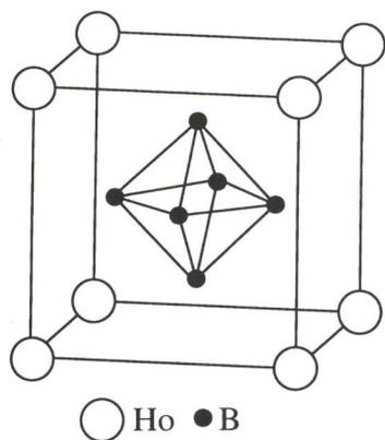
Fig. 3. The simple cubic crystal structure of HoB<sub>6</sub>.
