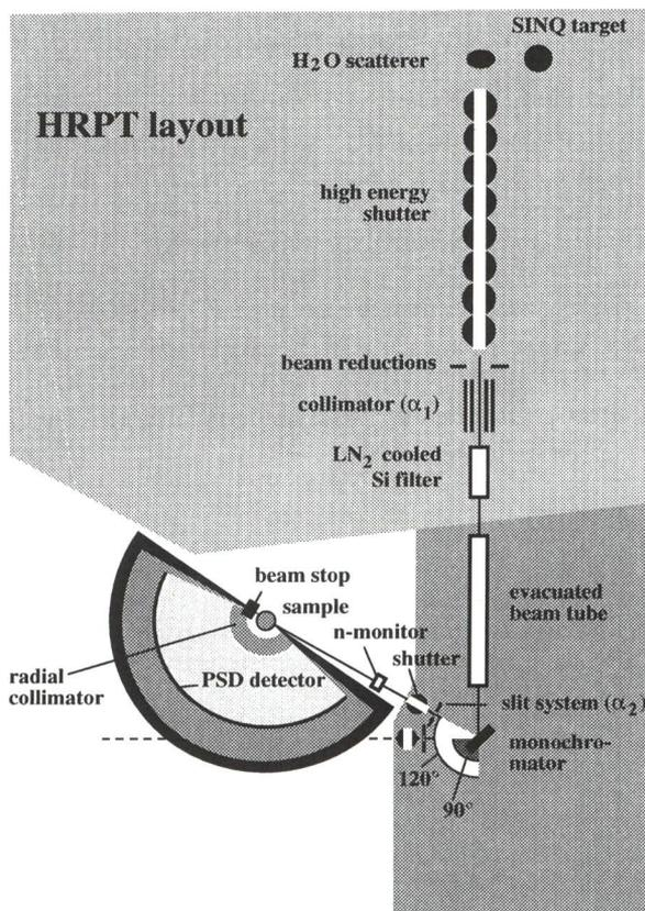
Fig.1. Layout of HRPT diffractometer at SINQ.
