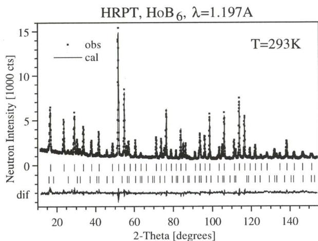
Fig. 4. Observed, calculated and difference HRPT neutron diffraction patterns ( $\lambda = 1.197$  Å, high-intensity mode) of HoB<sub>6</sub> at 293 K. Vertical bars indicate positions of nuclear Bragg peaks for HoB<sub>6</sub> (upper row) and for the impurity phase HoB<sub>12</sub> (lower row).
