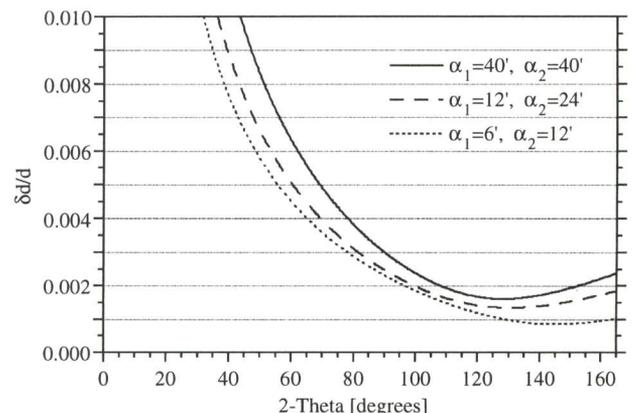
Fig.2. Measured resolution functions of HRPT for monochromator take-off angle  $120^\circ$  and sample diameter 10 mm (Si powder standard).
