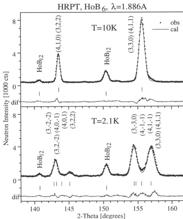
Fig. 5. High-scattering angle part of observed, calculated and difference HRPT neutron diffraction patterns ( $\lambda = 1.886$  Å, high-resolution mode) of HoB<sub>6</sub> at 10 and 2.1 K. Vertical bars indicate positions of nuclear Bragg peaks for HoB<sub>6</sub> (upper row) and for the impurity phase HoB<sub>12</sub> (lower row).
