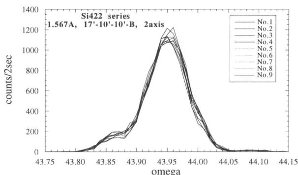
Fig. 2. Rocking curve of 422 reflection of 9-plates.
