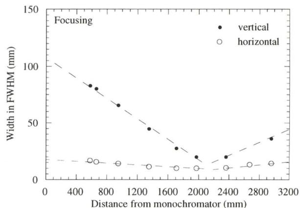
Fig. 4. Beam size as a function of the distance.
