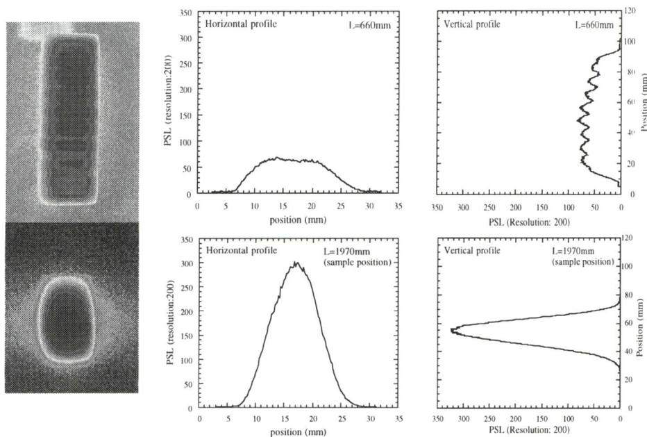
Fig. 3. Focusing effect of the bent monochromator.
