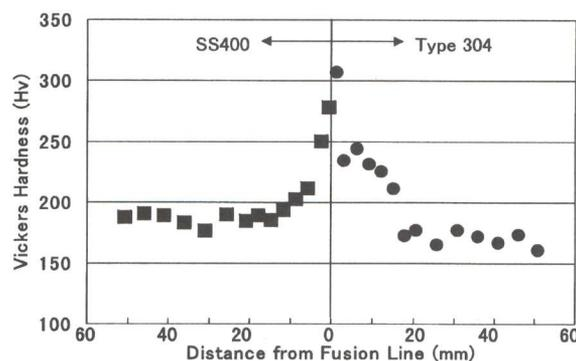
Fig. 4. Vickers hardness distribution after friction welding.
