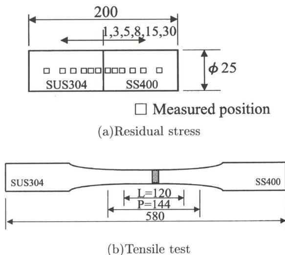
Fig. 1. Measurement point of the specimen(a) and dimensions of a specimen for tensile tests(b).
