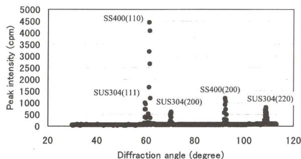
Fig. 2. Neutron diffraction pattern of friction welding boundary.
